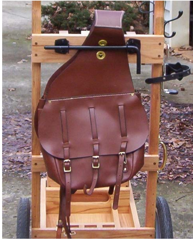
Figure 12, Back of cart detail showing location of Crane Bolt, Saddle Bags, Coat Hook and Carry Handle
